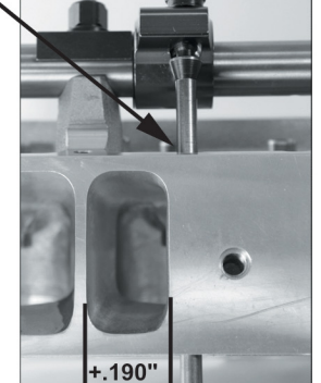
Port Width By Pushrod +.190" Wider Than Stock
